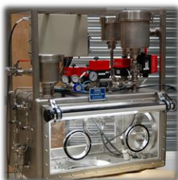
Client : Orano Project : Design and manufacturing of glove boxes for radioactive effluents management
